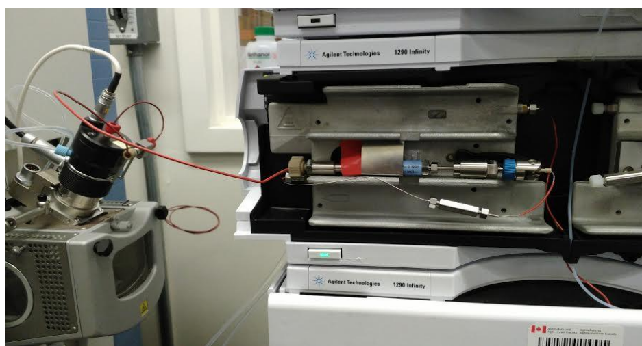
Figure 6- C18 column connected to the ESI source of the mass spectrometer
